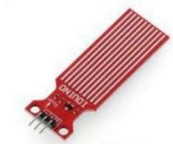
Gambar 5. Water level sensor
