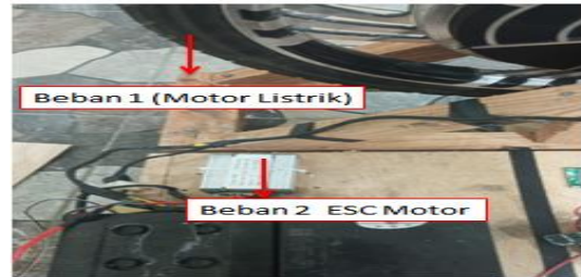
Image 5. Load circuit of the electric motorcycle wheel and the ESC module.
