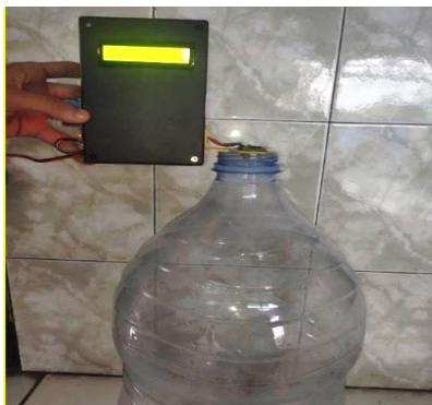
Figure 5 IoT-based Water Level Monitoring System Prototype
