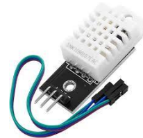
Image 4. DHT22 Temperature Sensor
