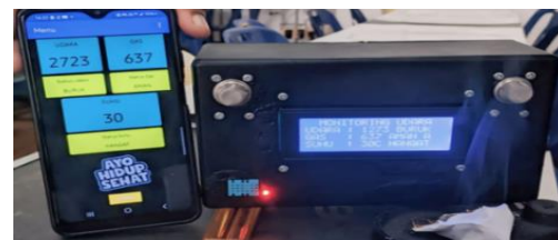
Image 2. Air Sensor Testing With Paper Waste Smoke
