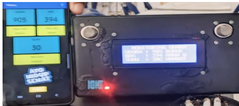
Image 3. Air Sensor Testing With Cigarette Smoke
