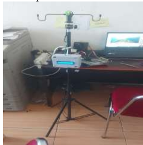
Image 3. Physical Form of the Infusion Water Volume Detector Device
