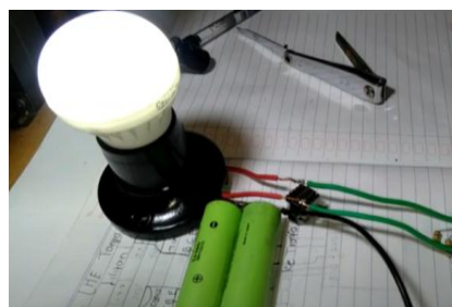
Figure 7. Joule thief test with a voltage of 7.4 VDC
