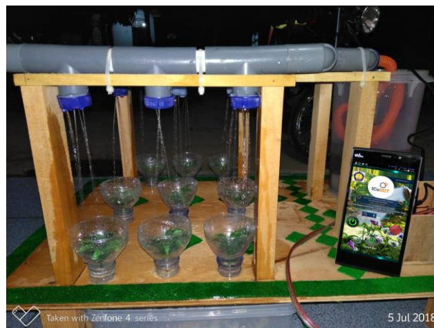
Image 5. Android-based Automatic Flower Watering System and Prototype Technical Testing
